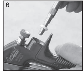
6. Remove Valve Seat.
