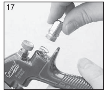
17. Replace Valve Spring and screw in Housing (10).
