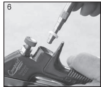
6. Remove Valve Seat.
