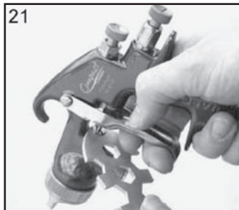
21. Adjust Needle Packing (4) with Spanner sufficient to seal but to allow free movement of needle. Lubricate with gun oil.
