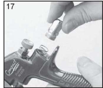
17. Replace Valve Spring and attach Housing (10).
