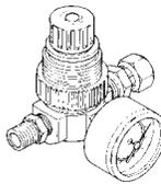
Use to maintain nearly constant outlet pressure despite changes in inlet pressure and downstream flow.
