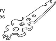
Contains all necessary tip, hose and nut sizes used on or with gun.
