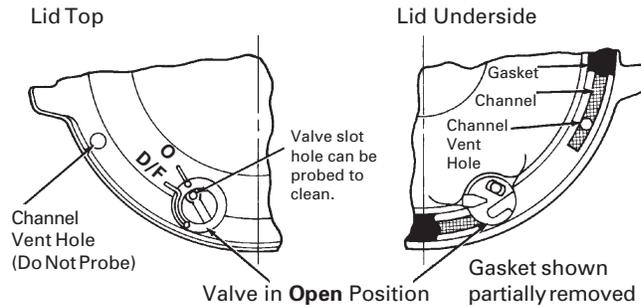
**Drip Free Mode "D/F"** - To operate in the drip free mode, rotate the valve with a screwdriver or coin so that the hole in the valve slot is aligned with the "D/F" on the lid. See Figure 3.
