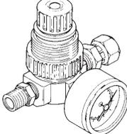
Use to maintain nearly constant outlet pressure despite changes in inlet pressure and downstream flow.
