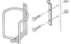
(1) Wall mount bracket included with GH-407. Holds standard paint cups, gravity feed guns and cups, and paint filters.
