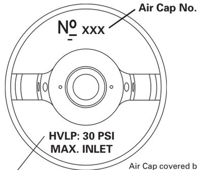
Maximum air pressure required to assure compliance of 10 PSI Max. Cap Pressure - this reading must be taken at the spray gun handle inlet fitting.
