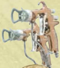
*The spray fan pattern is adjustable on the gun*
